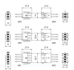
• Tinned brass, cylindrical terminals, plug male and socket female, for connections which is possible to connect to all the cables listed in "Section 9".
