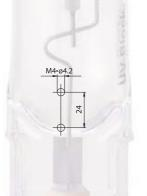
• Fixing of the lampholders pair by M4 screws to be inserted in the fixing holes with center distance 24 mm.
