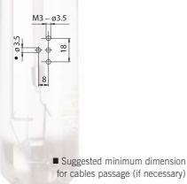
• Fixing of the lampholder using the holes diameter 3,5 mm with center distance 18 mm (if M3 screws are used, the head diameter should be less than 5,5 mm).
