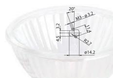
• Fixing of the lampholder by holes diameter 3,2 mm center distance 11,4 mm (if M3 screws are used, the diameter of the head must be less than 6 mm). During the fixing process the glass-holder spring must be positioned according to the drawing.
