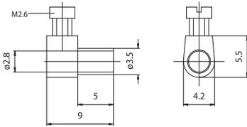
**204: Brass clamp** with screw to be used as device for ground connection, to be fixed in the hole of the metal support hamming the cylindrical part of the clamp.
