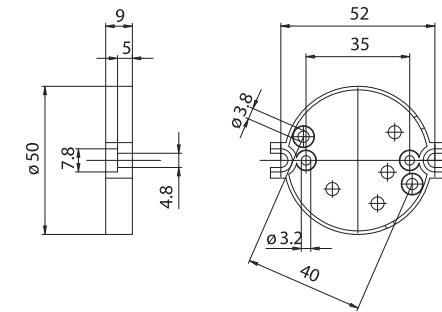
**227:** Closing base for double insulation in black PA66 20% G.F. V2, T140°C, with center distance 52 mm.
