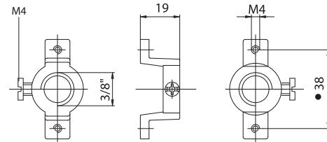
**230:** adapter, in white zinc-plated aluminium, with threaded hole 3/8" with center distance 38 mm, to fix the lampholder, and with screw for nipple-block.
