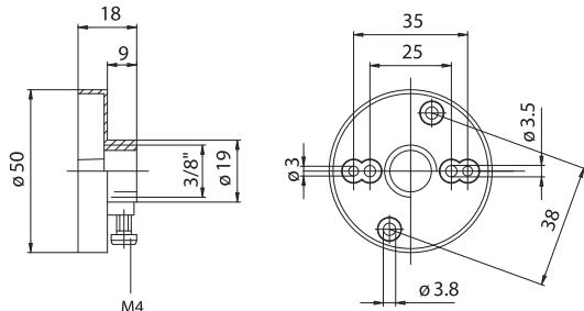
**228:** adapter with threaded hole 3/8", in black PA66 20% G.F. V2, T140°C, with screw for nipple-block.
