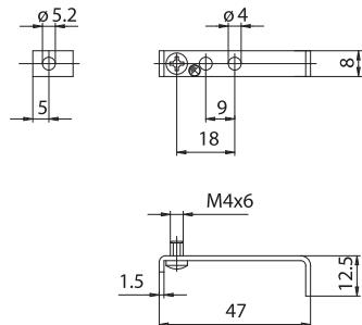
**209:** 90° bracket, in white zinc-plated iron, with hole diameter 5,2 mm and earth-screw, for fixing on structures with threaded holes M4.
