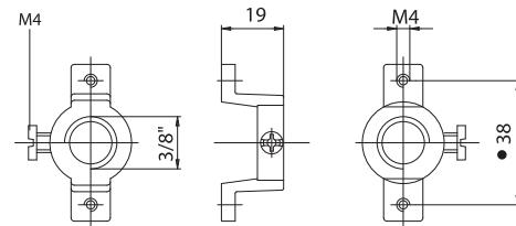
**230:** adapter, in white zinc-plated aluminium, with threaded hole 3/8" with center distance 38 mm, to fix the lampholder, and with screw for nipple-block.
