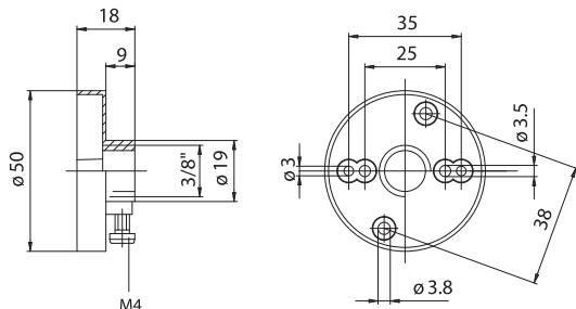
**228:** adapter with threaded hole 3/8", in black PA66 20% G.F. V2, T140°C, with screw for nipple-block.
