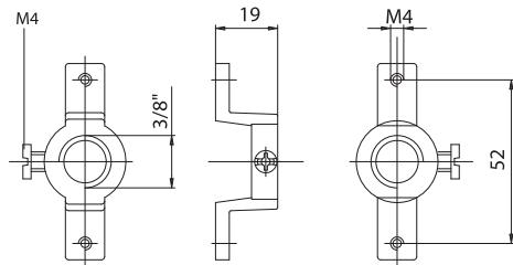
**231:** adapter, in white zinc-plated aluminium, with threaded hole  $3/8''$  with center distance 52 mm, to fix the lampholder, and with screw for nipple-block.
