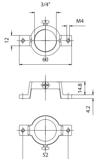
**233:** adapter, in white zinc-plated aluminium, with threaded hole  $3/4''$  with center distance 52 mm, to fix the lampholder, with screw for nipple-block.
