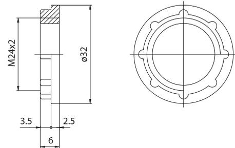
**279:** threaded adapter for very low tension lampholders with external thread M24 x2.
