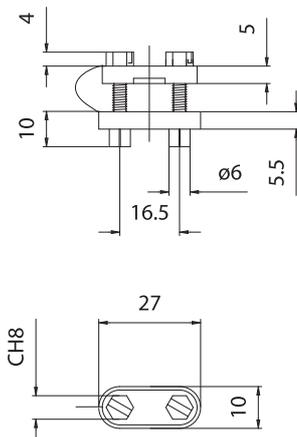
**760: Cable clamp** in natural PA66 T-20 +T125°C suitable to clamp cables with diameter between 3 and 10 mm.
