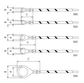
• Brass eyelet terminals, which is possible to connect to all the cables listed in "Section 9" (normally used for the earth conductors).
