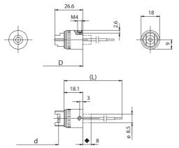
◆ Maximum jut of the steatite body during lamp insertion
