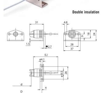
◆ Maximum jut of the steatite body during lamp insertion
