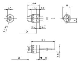
◆ Maximum jut of the steatite body during lamp insertion
