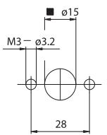
■ Insertion hole of the porcelain body during lamp insertion
