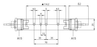
▲ Dimension without inserted lamp in the lampholder ◆ Maximum jut of the porcelain body during lamp insertion
