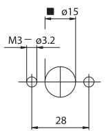
■ Insertion hole of the porcelain body during lamp insertion
