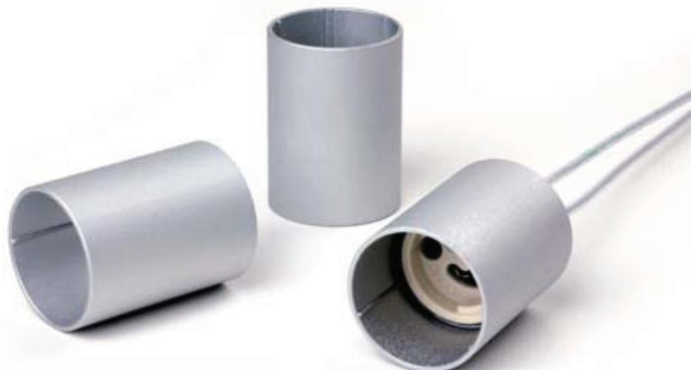
**A42CB:** version of the lampholder A42 with back central exit of the cables and aesthetical cover in sand-blasted and anodized aluminium (for the cover ref. art. 496/42B).
