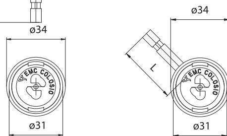
**A85LCQ:** version of the lampholder A85 with lateral exit of the cables and aesthetical cover in polished aluminium (for the cover ref. art. 496L/27Q).
