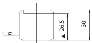
**A85CQ:** version of the lampholder A85 with back central exit of the cables and aesthetical cover in polished aluminium (for the cover ref. art. 496/27Q).
