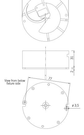
. Fixing of the device by M3 screws to be inserted in the holes at center distance 77 mm.
