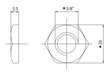
**M16:** nut, in aluminium, hexagonal 26 mm, with threaded hole 3/8".
