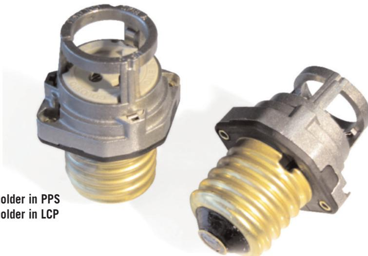
**M204/A91:** Adapter with cap E39/39 (Mogul base) with lampholder PGZ12, our code A91, with temperature of the part screw shell limited to T200°C.
