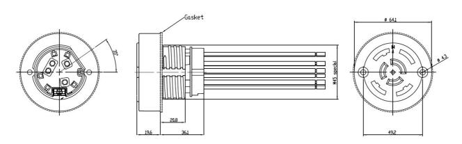
M400-: 3 Poles (4 Ways) "Power" + 4 Poles (5 Ways) "Signal" photocontrol plug-in locking type socket (Nema Socket), built up with a main socket device (code M400C-) and a part movable wired connector (code M400M-)
