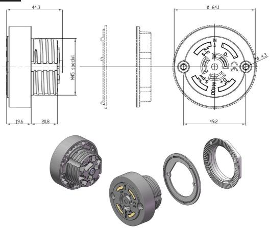
**M400C-:** Part socket of the 3 Poles (4 Ways) "Power" + 4 Poles (5 Ways) "Signal" photocontrol plug-in locking type socket (Nema Socket), to be coupled with the part connector M400M-, to be fixed using two M4 screws (front fixing) or using the nut 2026F (rear fixing) interposing, between the device and the fixing structure, the gasket 2029F.
