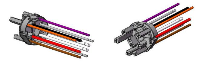
M400M-: Part Connector of the 3 Poles (4 Ways) "Power" + 4 Poles (5 Ways) "Signal" photocontrol plug-in locking type socket (Nema Socket) to be coupled with the part socket M400C-, wired with cables from section 0.35 mm² (or AWG 22) to section 1.00 mm² (or AWG 18).
