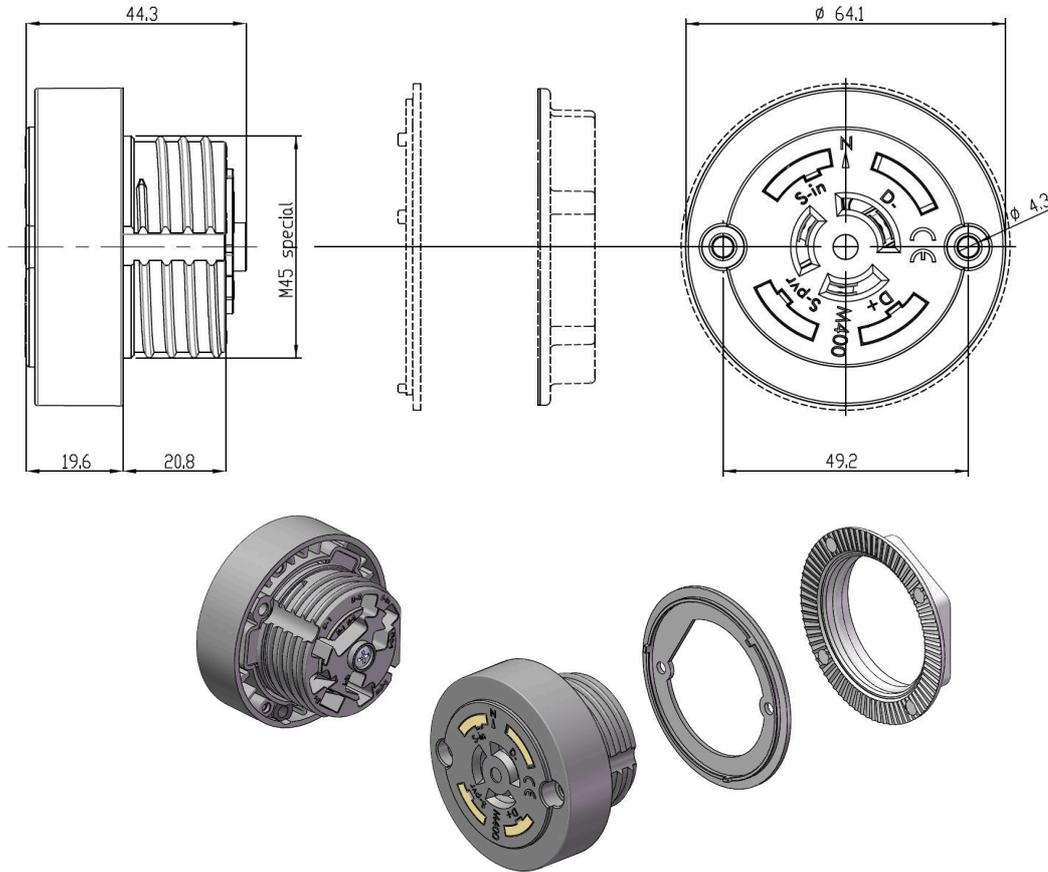
**M400C-**: Part socket of the 3 Poles (4 Ways) "Power" + 4 Poles (5 Ways) "Signal" photocontrol plug-in locking type socket (Nema Socket), to be coupled with the part connector M400M-, to be fixed using two M4 screws (front fixing) or using the nut 2026F (rear fixing) interposing, between the device and the fixing structure, the gasket 2029F.
