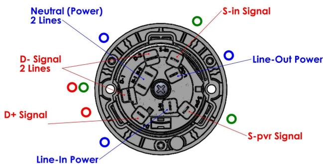
Wiring diagram / back view
