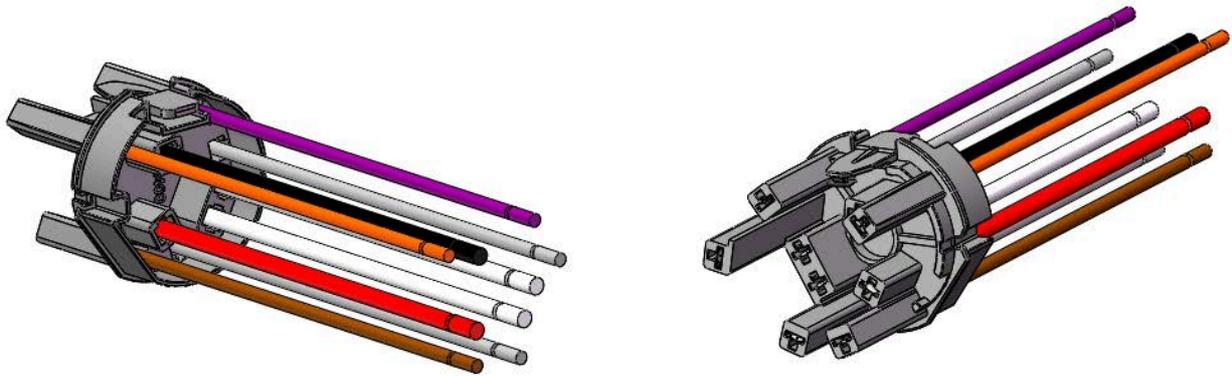
**M400M-**: Part Connector of the 3 Poles (4 Ways) "Power" + 4 Poles (5 Ways) "Signal" photocontrol plug-in locking type socket (Nema Socket) to be coupled with the part socket M400C-, wired with cables from section 0.35 mm<sup>2</sup> (or AWG 22) to section 1.00 mm<sup>2</sup> (or AWG 18).
