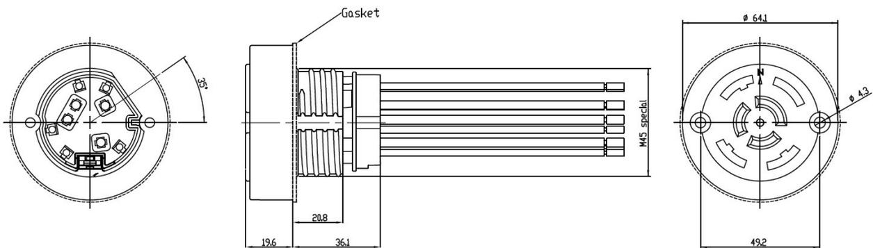
**M400-**: 3 Poles (4 Ways) "Power" + 4 Poles (5 Ways) "Signal" photocontrol plug-in locking type socket (Nema Socket), built up with a main socket device (code M400C-) and a part movable wired connector (code M400M-)
