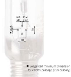
• Fixing of the lampholder using the holes diameter 3,2 mm with center distance 18 mm.
