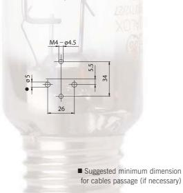
• Fixing of the lampholder using the holes diameter 4,2 mm with center distance 34 mm.
