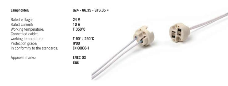
Single-conductor flexible connecting cables crimped to the lampholder:
