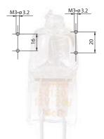
• Eventual fixing of lampholders P70 and P70D by slots, width 3,2 mm, with center distance from 16 to 20 mm.
